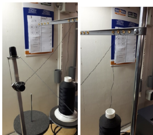
The proper way the treaddirection into te machine
